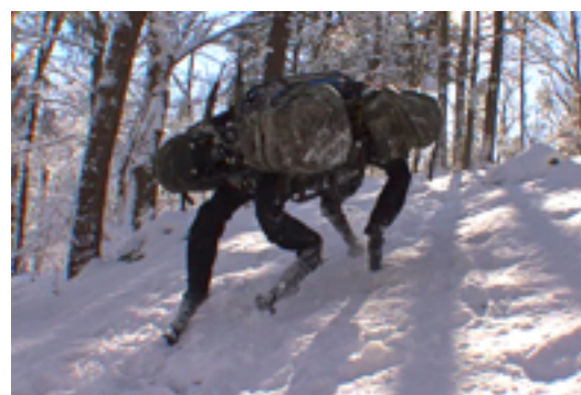
Boston Dynamics’ BigDog rough-terrain robot walks, runs, climbs and carries heavy loads. It’s 3 ft. long, 2.5 ft. tall, weighs 240 lbs. and can travel 12.8 miles without stopping or refueling. Update: A larger BigDog will be deployed in 2012.
